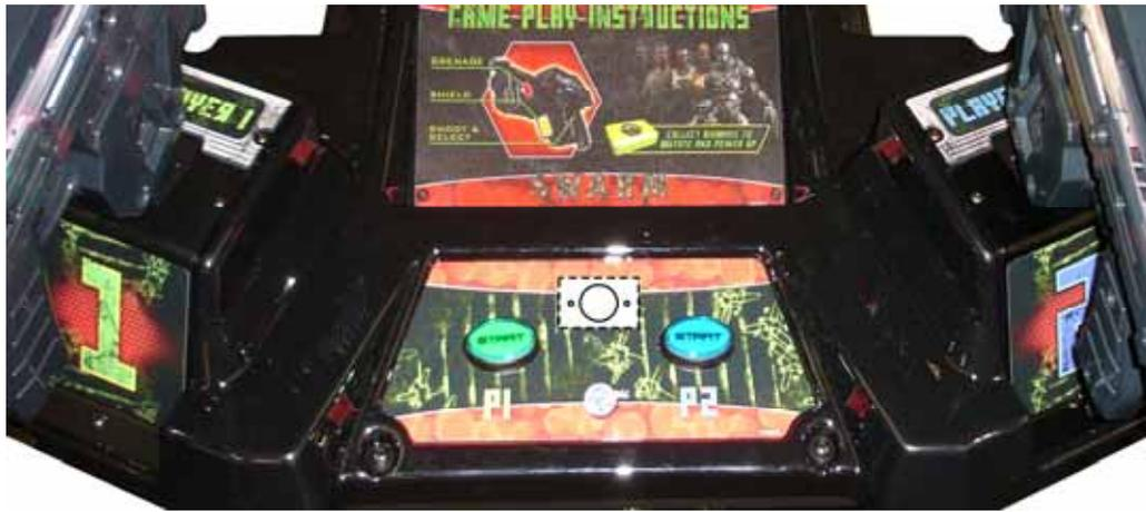
Figure 3. Button Template Placement
