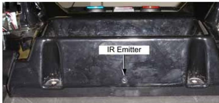
*Figure 1. Suggested IR Emitter Placement*
