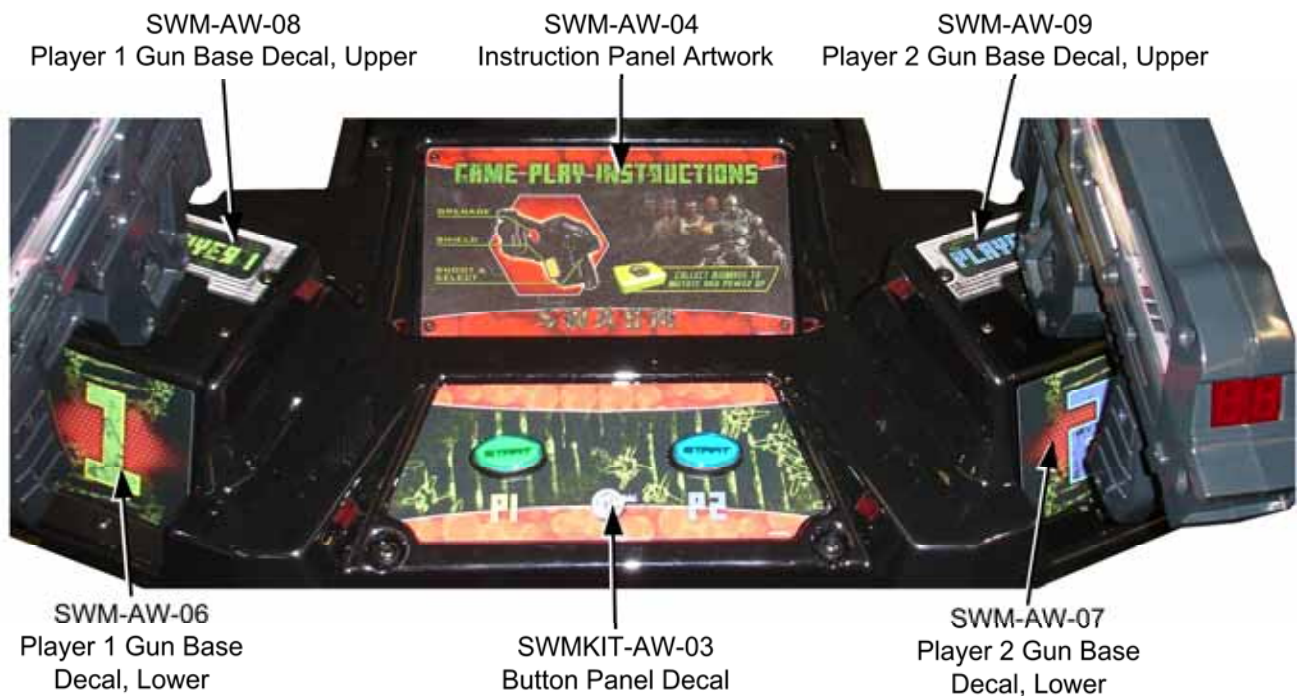
Figure 4. Control Panel Artwork Placement
