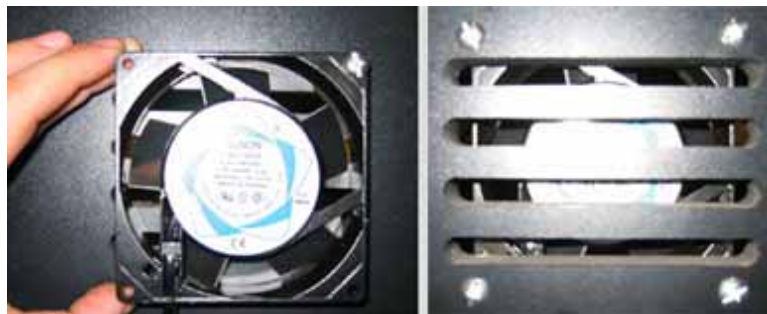
Figure 7. Installing the Ventilation Fan
