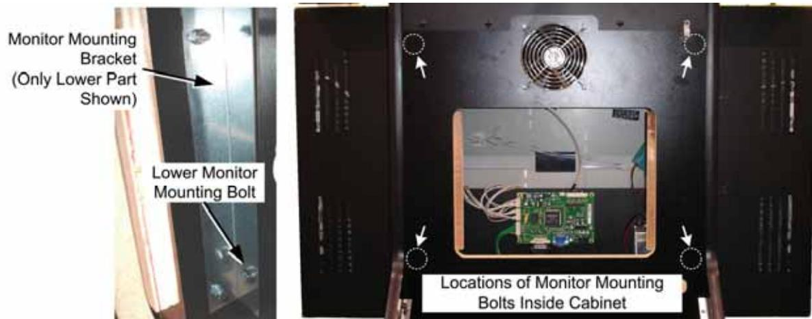
Figure 2. Monitor Mounting Bolts
