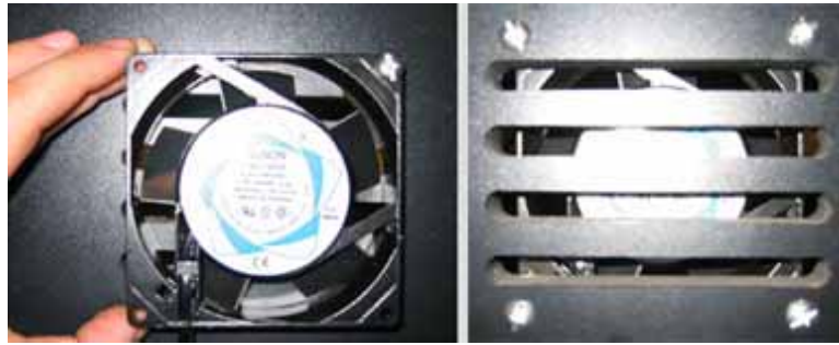
Figure 3. Installing the Ventilation Fan
