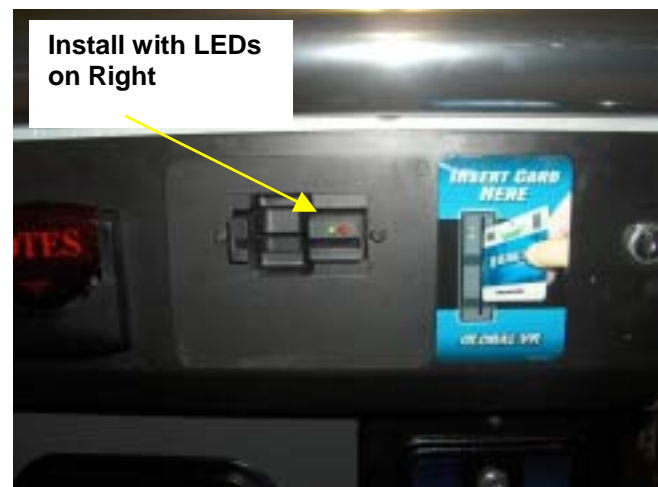
Figure 5. SmartCard Reader and Artwork Installed
