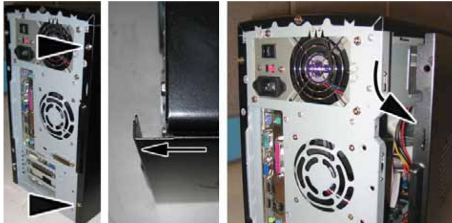
2. Remove the plastic feet from the computer case by using pliers to squeeze the tops of the feet inside the case, while pulling the feet off from the outside.
