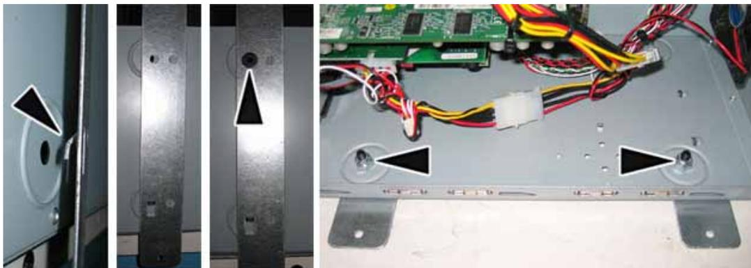
6. When finished, the two screws with nuts should be closest to the outside edge of the computer chassis, with the bracket tabs hooked into the holes closest to the motherboard, as shown in the last part of the picture above. Re-install the side panel on the computer.
