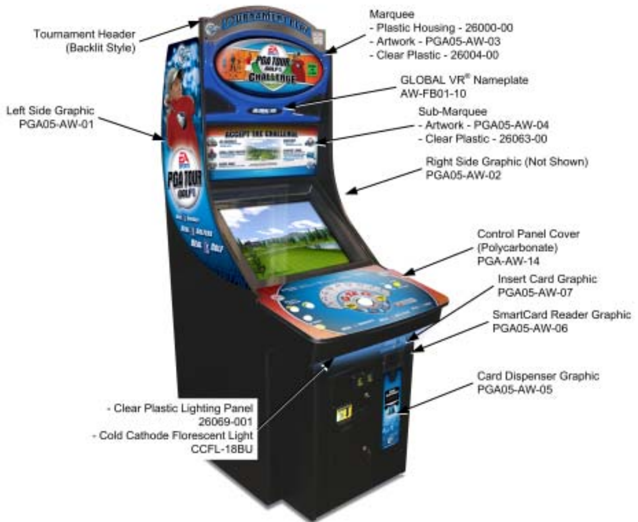
Figure 39. Cabinet Artwork and Formed Components
