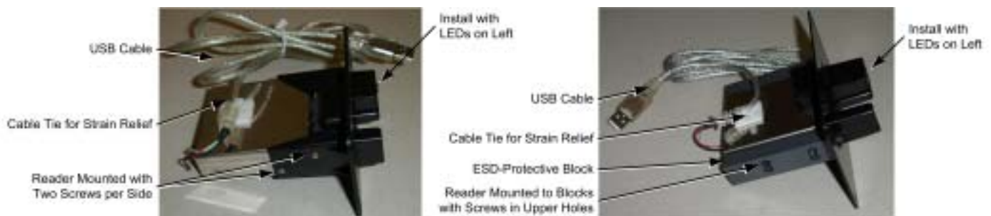
Figure 3. SmartCard Reader Assembly
