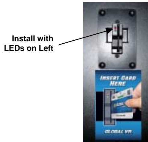
Figure 4. SmartCard Reader and Artwork Installed
