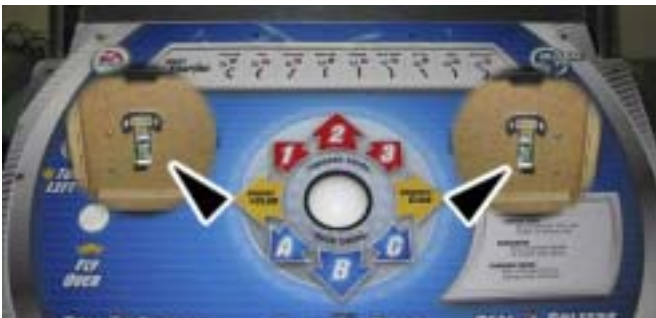
Figure 2 – Releasing the Latches Under the Control Panel
