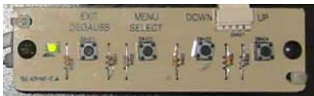
Figure 25 – Monitor Control Panel
