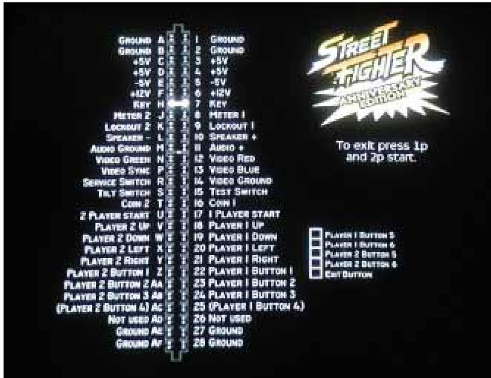
Figure 14. JAMMA Test Screen
