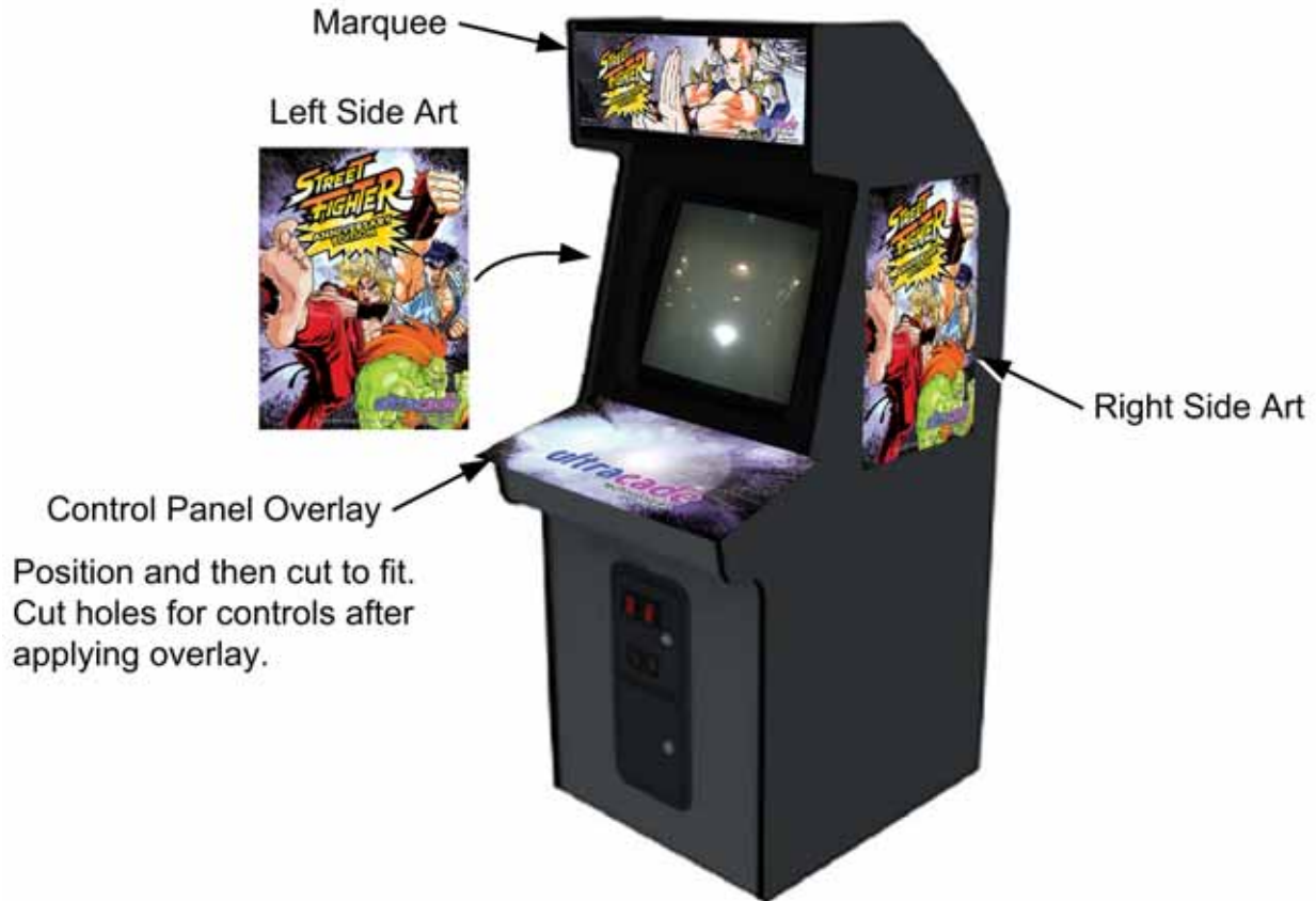
Figure 9. Applying Cabinet Artwork
