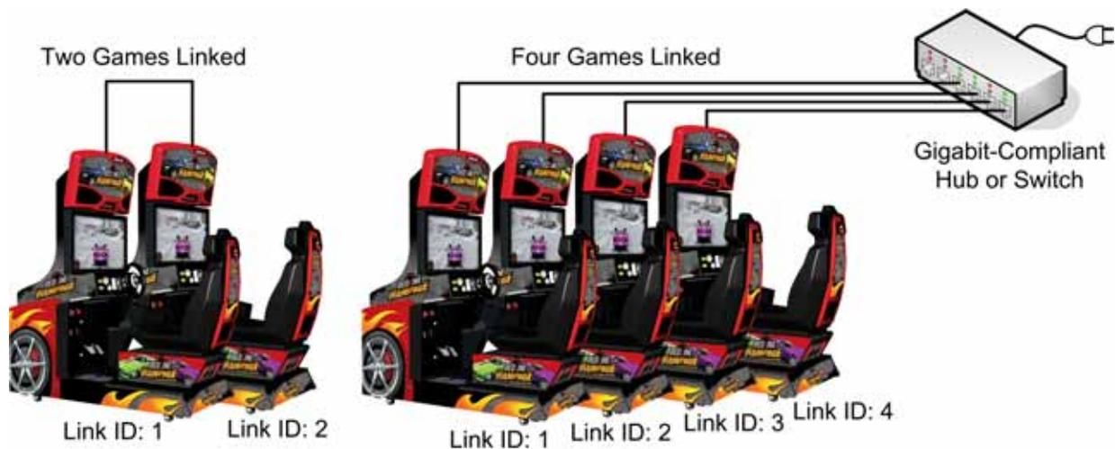
Figure 1. Linking Cabinets
