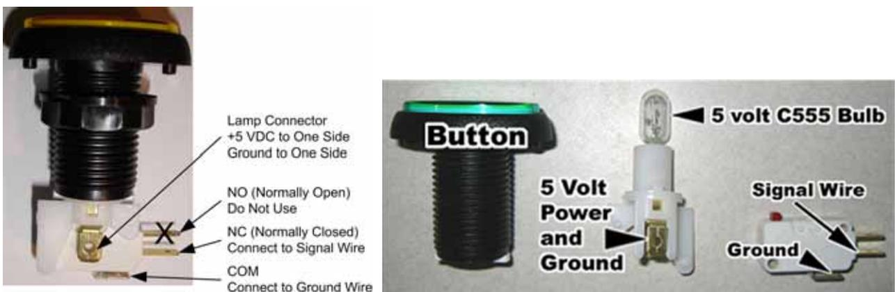
*Figure 5. Lighted Button Connectors*
