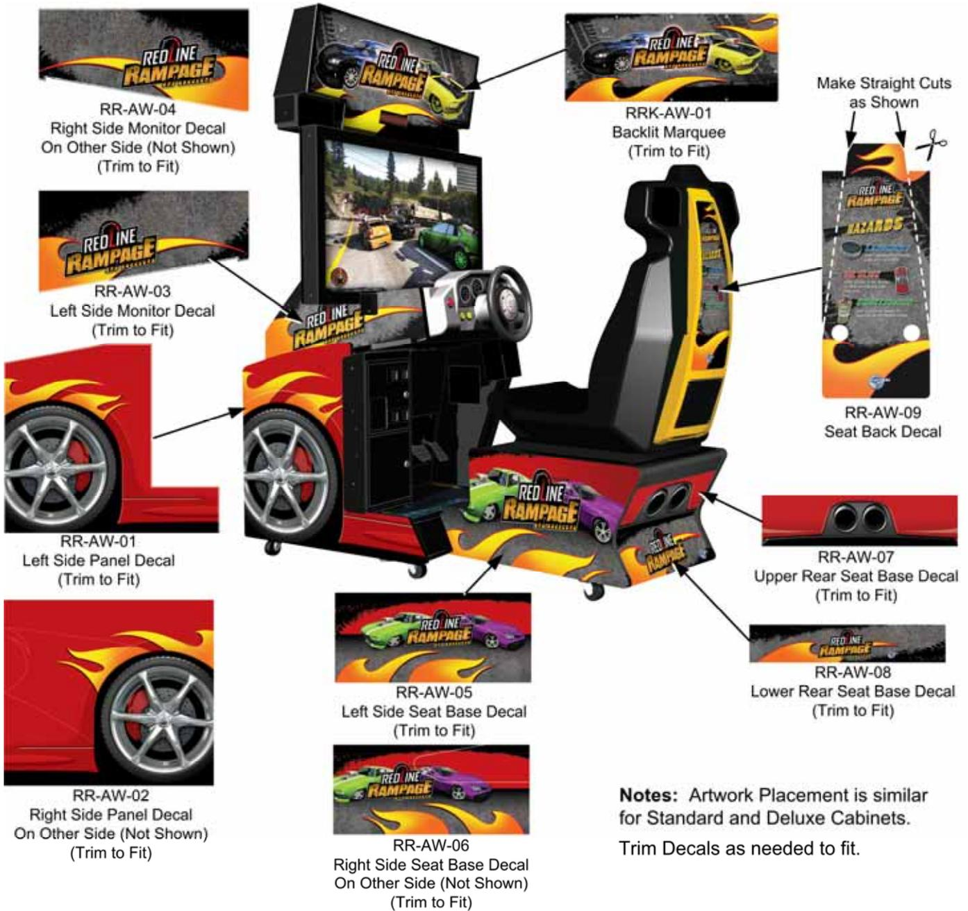
Figure 11. Artwork Placement on Twisted Cabinet
