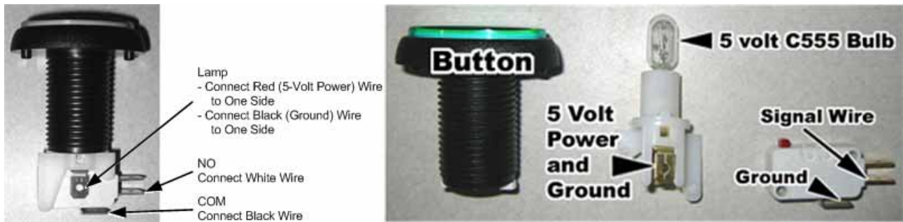
Figure 6. Button Assembly
