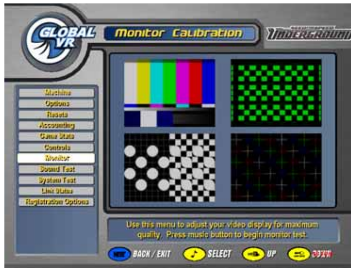
Figure 17. Monitor Calibration Test Screen
