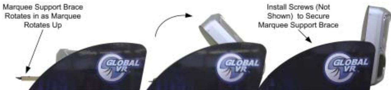
Figure 5. Setting up the Marquee
