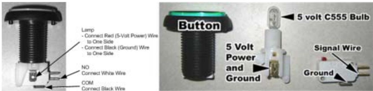
Figure 30. Replacing Button Lamps
