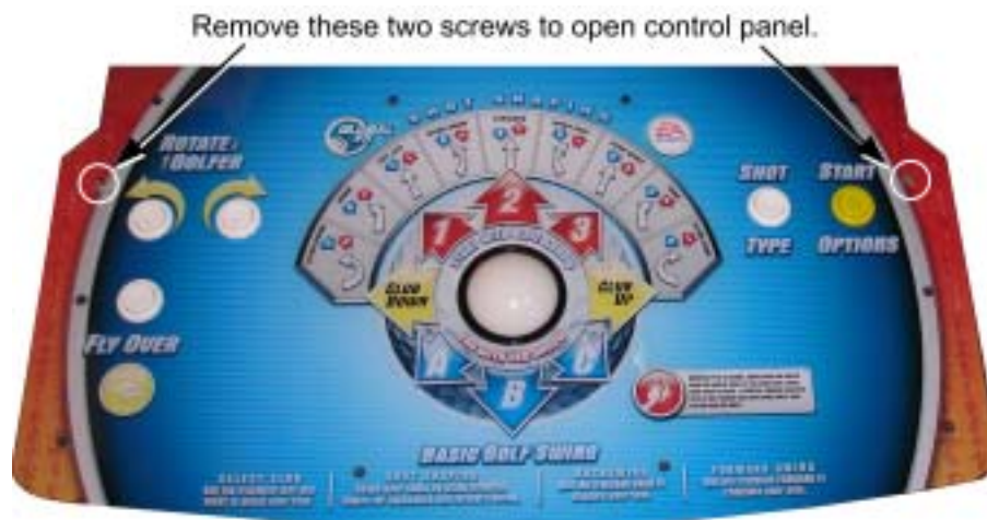
Figure 5. Opening the Control Panel
