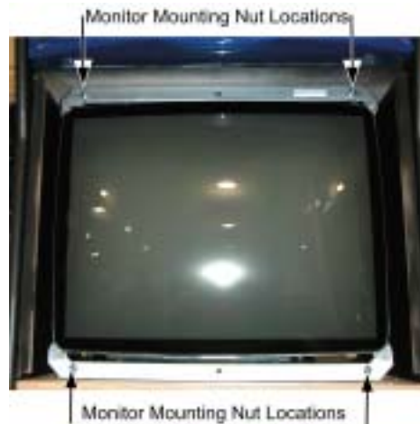
Figure 8. Monitor Mounting Nut Locations
