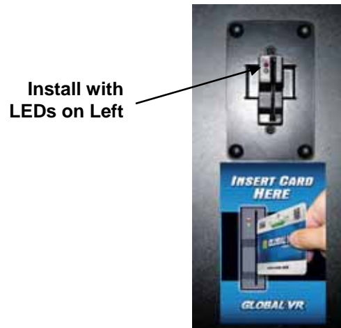
Figure 4. SmartCard Reader and Artwork Installed
