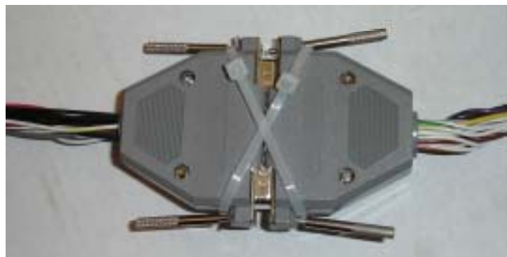
Figure 7. Securing the DB37 Connectors
