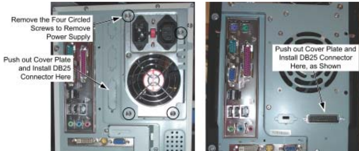
Figure 2. Installing the DB25 Connector on PC Rear
