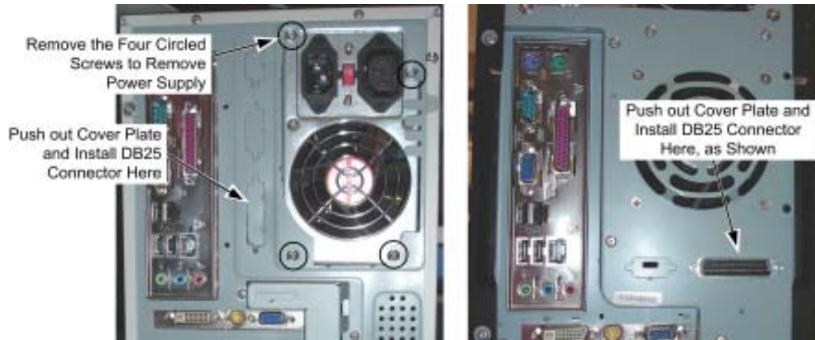
Figure 2. Installing the DB25 Connector on PC Rear
