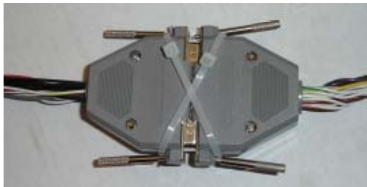
Figure 5. Securing the DB37 Connectors
