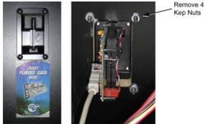
*Figure 4. Removing the Old Card Reader*
