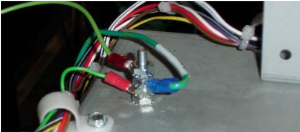
Figure 3. Coin Vault Ground Lug
