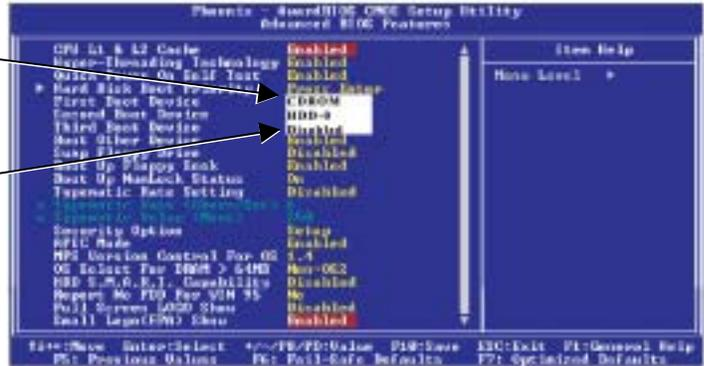
**Note:** If a floppy drive is installed, set **First Boot Device** to **Floppy**, **Second Boot Device** to **CDROM**, and **Third Boot Device** to **HDD-0**.
