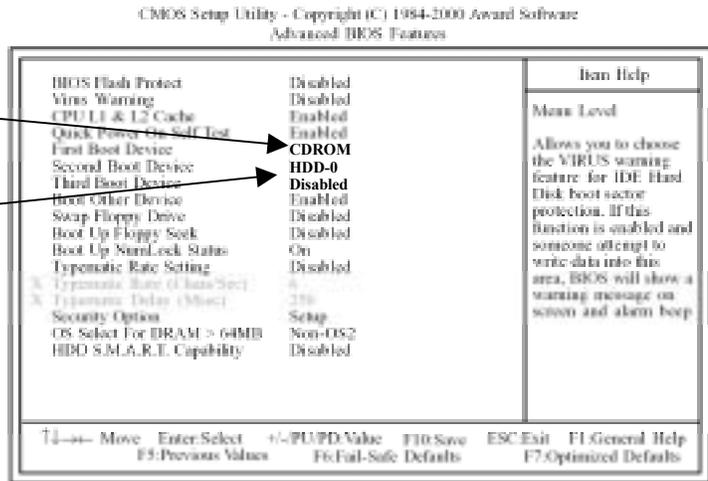
7. Set **Second Boot Device** to **HDD-0** and **Third Boot Device** to **Disabled** the same way. Press **ESC** to go back to the Main Menu.
