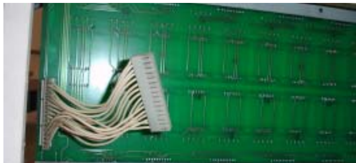
Figure 2. 16-Pin Connector from LED Board
