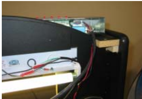
Figure 2. Route Harness Around Florescent Fixture
