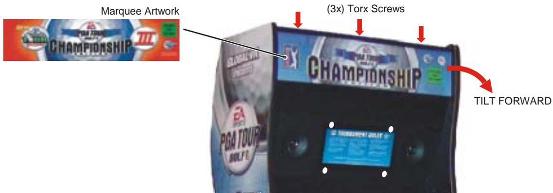
*Figure 2. Installing New Cabinet Artwork*
