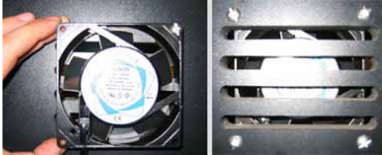
Figure 5. Installing the Ventilation Fan
