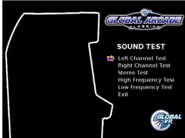
The Sound Test menu lets you test the stereo sound. When you press **Player-1 Button-1** to select a test from the menu, you will hear the sounds described below, and see a graphic indicating which speaker(s) should be playing the sound:
