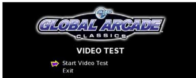
The Video Test displays screens that can be useful when making adjustments to the monitor. After selecting **Start Video Test**, press **Player-1 Button-1** repeatedly to cycle through Red, Green, Blue, Color Bars, and Pin Cushion screens.
