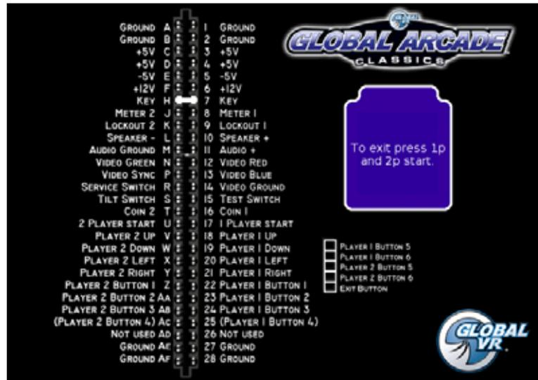
The JAMMA Test screen lets you test each JAMMA connection for the player controls, coin mech, and **Service** button. The buttons that do not use the JAMMA harness are also shown on the screen.
