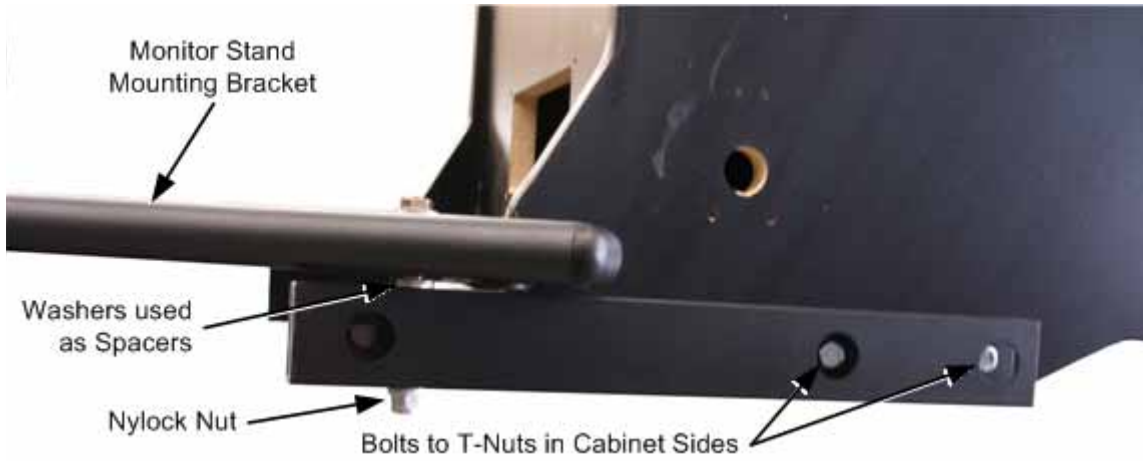
Figure 3. Cabinet and Mounting Bracket, Side View
