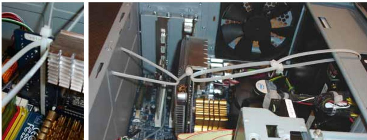
2. Observe how the cable ties are arranged in the picture above. The goal is to put equal tension on both sides of the video card. This will prevent the video card from moving up and down when the computer is upright in the cabinet, and the cabinet is jostled during shipping.
