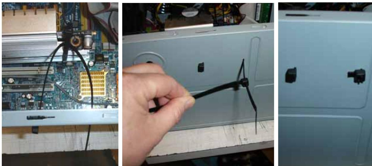
3. Carefully tighten the ties on both sides of the video card so that there is equal tension on both sides. Make sure the video card remains perpendicular to the motherboard.
