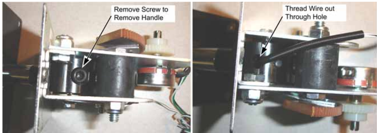
Figure 17. Replacing the Throttle Handle
