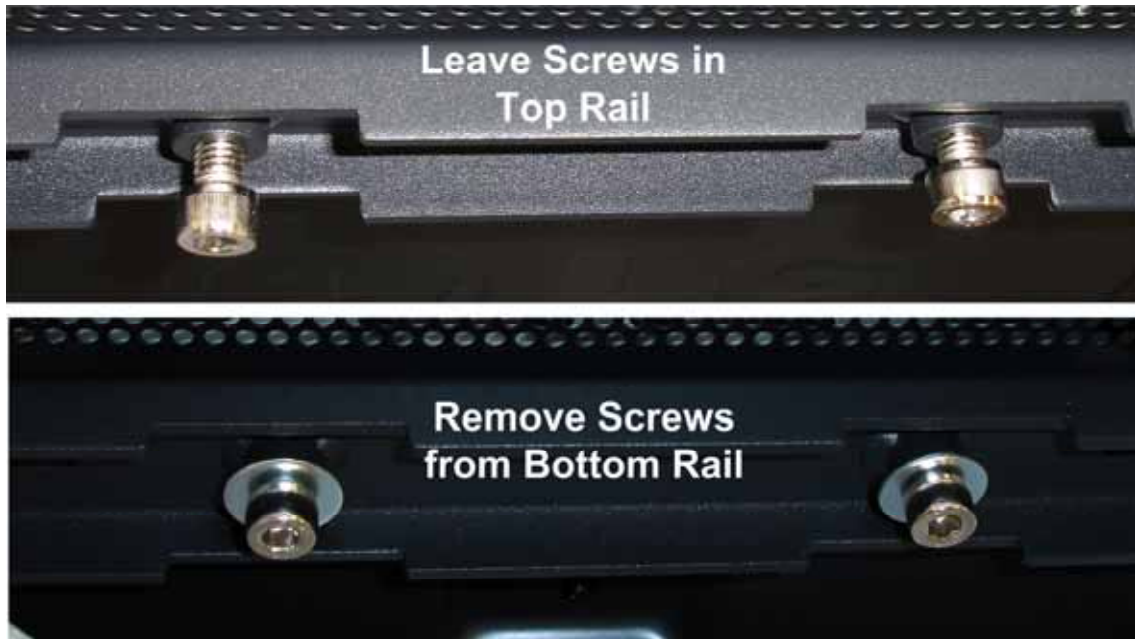
Figure 7. Top and Bottom Mounting Screws
