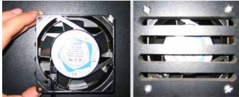
Figure 4. Installing the Ventilation Fan
