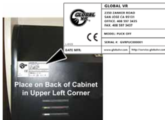
Figure 12. Applying the Serial Number Label
