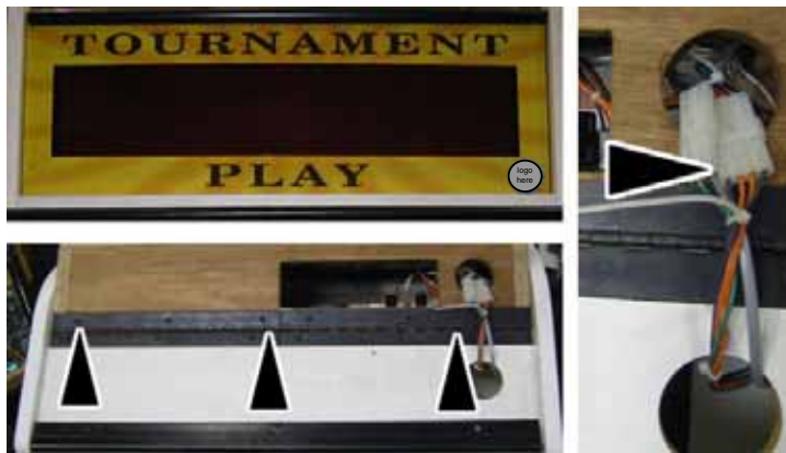
Figure 2. Removing Old Tournament Header.
